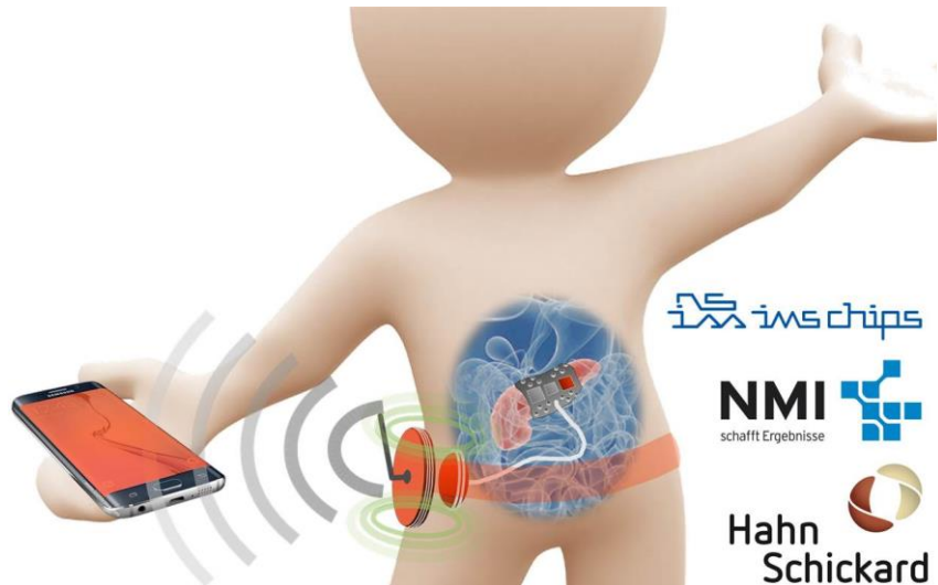
Abb. 1: Schematic display of the intelligent implant system consisting of a flexible, functionalized electrode mat that is attached to the pancreas, a power management and data communication buoy implanted directly beneath the skin, a belt-worn external unit and an Android device for data display and function control.
