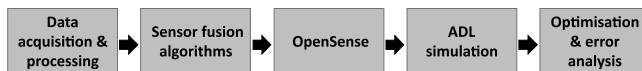
Figure 2: Method overview. IMU and MoCap data were processed to create personalised biomechanical models. Orientation estimates based on IMU data and sensor fusion algorithms were used in OpenSense to animate biomechanical models in ADL simulations. After parameter optimisation, IMU-based joint angle estimates were compared to MoCap.
