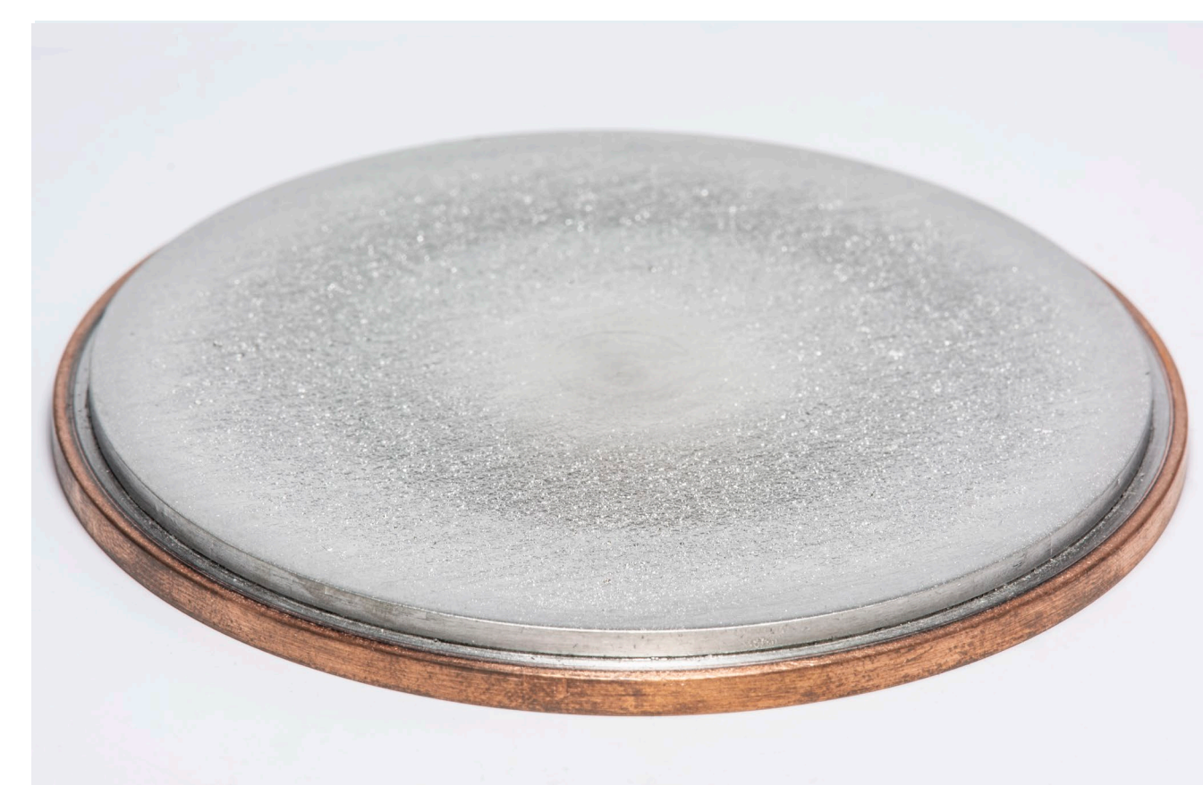
Fig.2: Ceramic sputtering target reactively bonded to a copper back plate (left), Stress sensor joined with Zr/Si/Al-RMS (right, cf. Fig.1)
