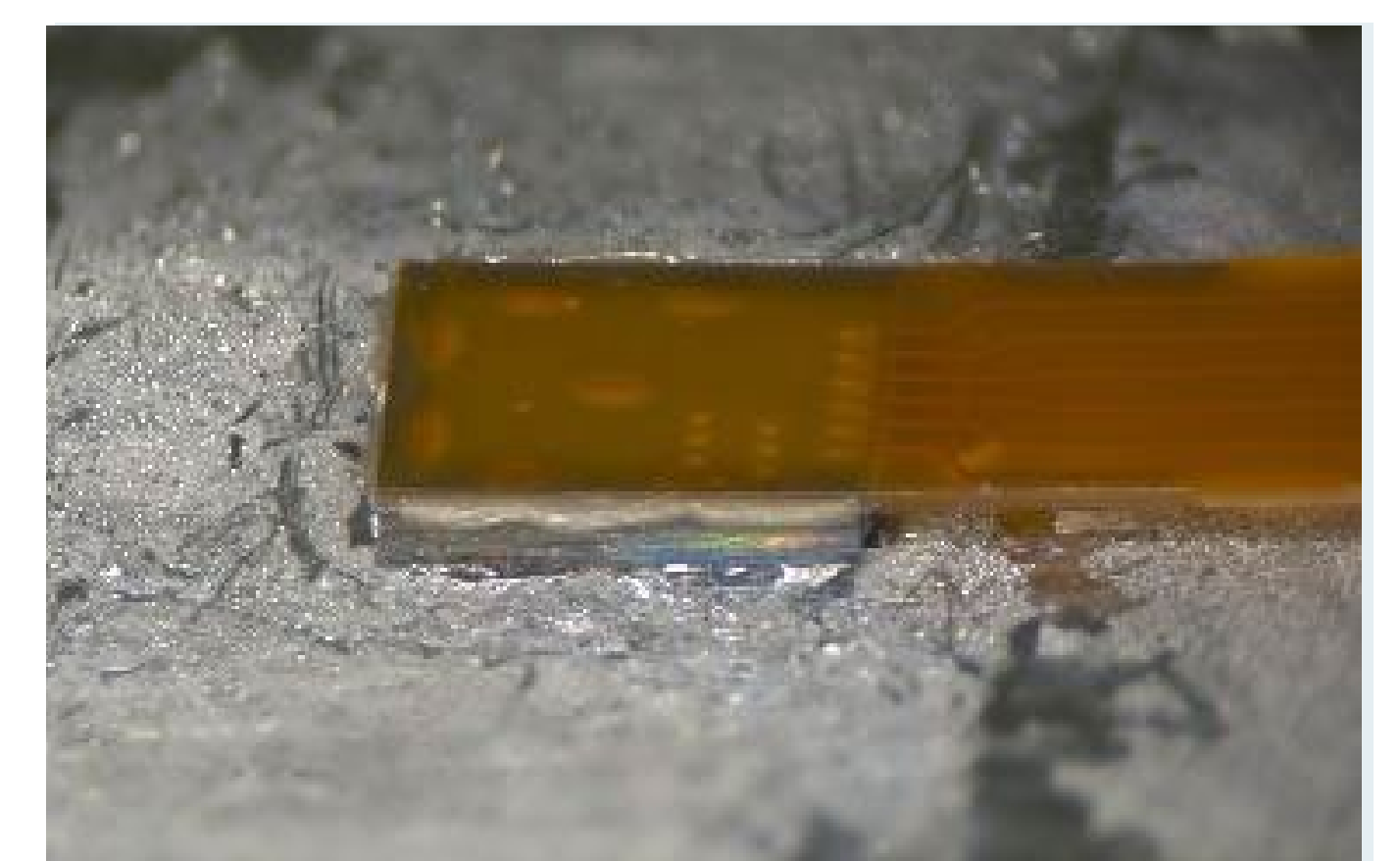
Fig.2: Ceramic sputtering target reactively bonded to a copper back plate (left), Stress sensor joined with Zr/Si/Al-RMS (right, cf. Fig.1)
