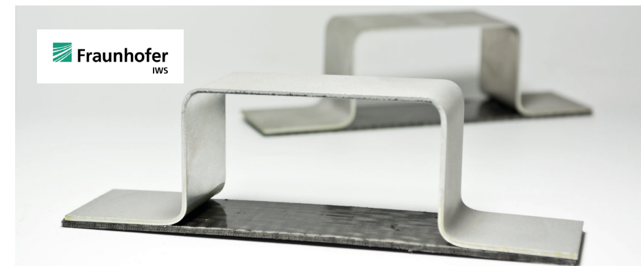
Hybrid joining of CFK with aluminium
