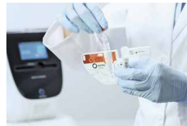
The fully automated Rhonda rapid PCR test system consists of an analyzer with a test cartridge. Source: Christian Eichenauer, scinelion
