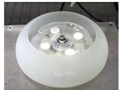
Fig. 2: Filters are integrated into the filter chambers by thermal bonding. The receptacle can be connected to a larger vessel for storage of larger fluid volumes.
