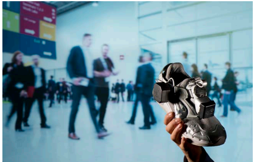
Fig. 1: The inertial sensor unit is mounted at the front of the shoe, the harvester at the side.
