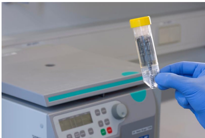
The LabTube cartridge and a table-top laboratory centrifuge as processing device.
