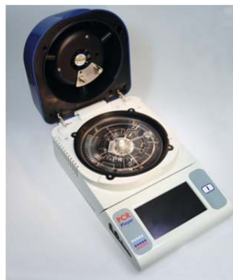
Fig. 1: LabDisk player with LabDisk for detection of respiratory pathogens.
