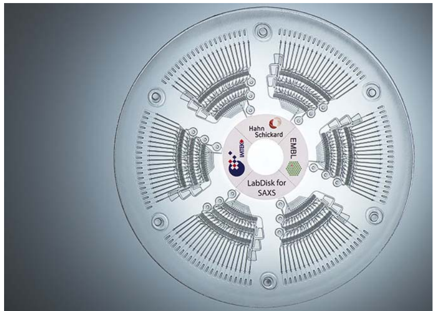
Fig. 1: SAXSDisk: Protein structure screening from only 2.5 µl protein volume.
