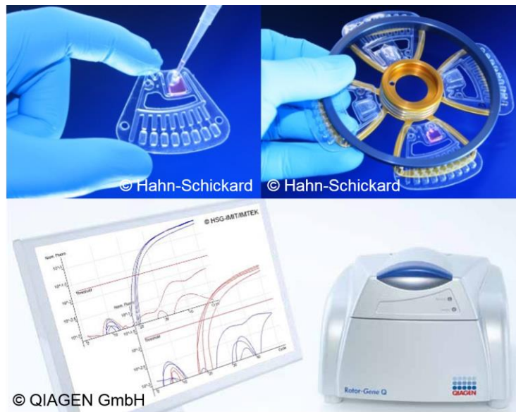
Fig. 1: One pipetting step for sample insertion. Here, four GeneSlices can be processed per run. Proof-of-concepts showed cross-contamination free amplification in a standard Rotor-Gene Q.
