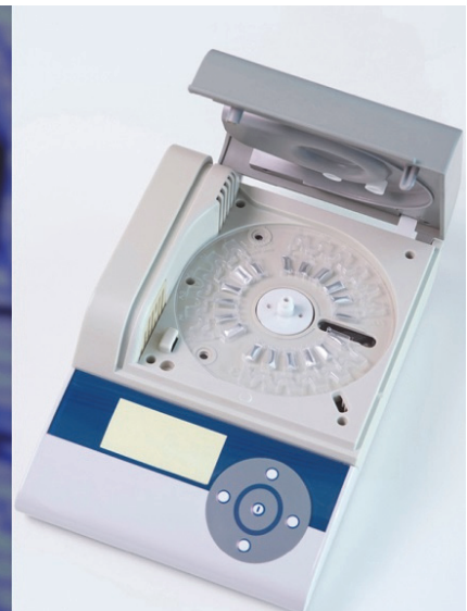
The LabDisk (with pre-stored buffers in stickpacks) and LabDisk Player
