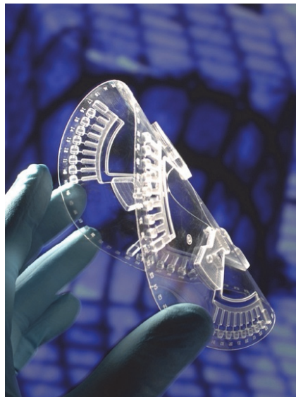
The LabDisk (with pre-stored buffers in stickpacks) and LabDisk Player
