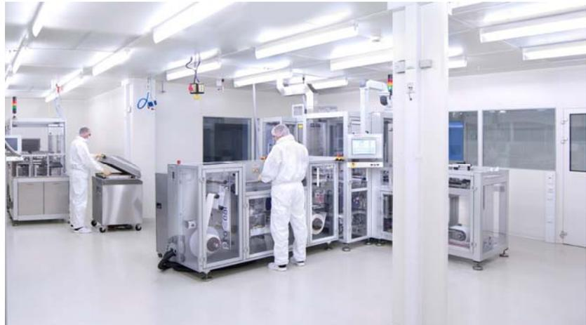
**Fig. 1:** Adaptable machine concept for up to 200.000 LabDisks / year (single shift). The operation of the pilot line in a clean room following the category 10,000 (ISO 7) guarantees optimum quality of the produced prototypes. Credit: Atelier Lünig for Harro Höfliger.
