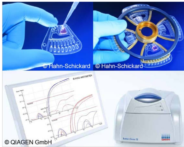
Fig. 1: One pipetting step for sample insertion. Here, four GeneSlices can be processed per run. Proof-of-concepts showed cross-contamination free amplification in a standard Rotor-Gene Q.
