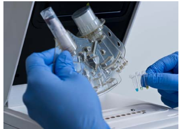
LegionellaSlice XL cartridge with detachable PCR tubes that are transferred to a thermocycler for analysis
