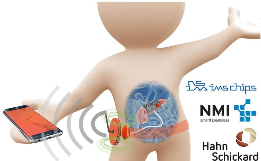
**Abb. 1:** Schematic display of the intelligent implant system consisting of a flexible, functionalized electrode mat that is attached to the pancreas, a power management and data communication buoy implanted directly beneath the skin, a belt-worn external unit and an Android device for data display and function control.
